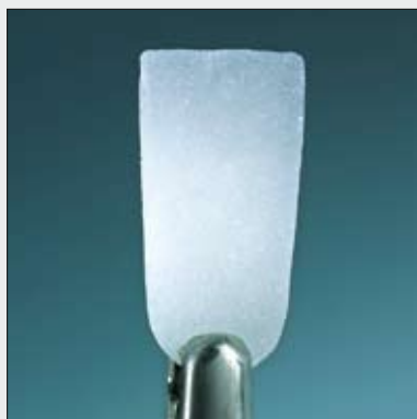
Fig. 2: Firing sample after furnace temperature too low
