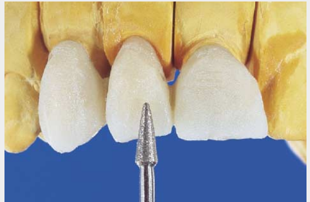
8. Grind the bridge lightly using a diamond bur (suitable diamonds see 4 page 23).
