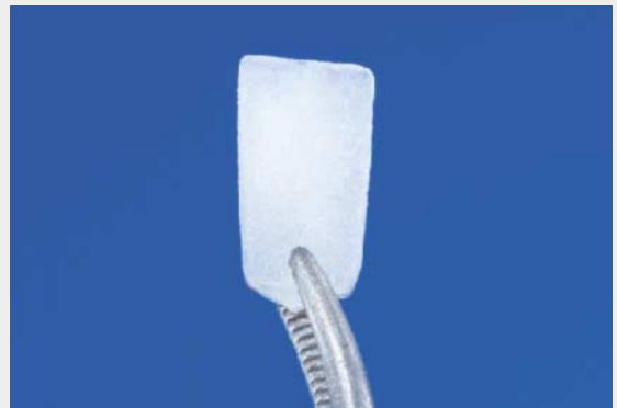
Fig. 1a: Bake specimen, temperature too low.
